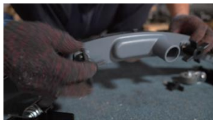
Step 2: Fix the plastic components on the cast aluminum base plate of the squeegee;
