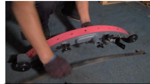
Step 3: Align the holes of the rear rubber strip with the plastic components of the squeegee to the protrusions;
