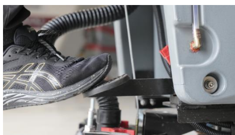
Step 1: Lightly step on the foot lever and put down the scrubber;
