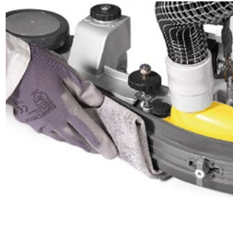
To ensure a perfect drying, the suction hose and the squeegee rubber blades must be cleaned at the end of any cleaning operation. The squeegee can be lifted to quickly clean the rubber blades
