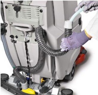
To ensure a perfect drying, the suction hose and the squeegee rubber blades must be cleaned at the end of any cleaning operation. The squeegee can be lifted to quickly clean the rubber blades
