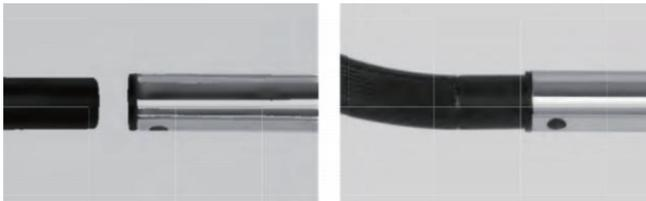
Connect the corresponding hose with the suction port of the machine and tighten it clockwise.
